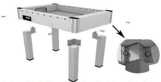
Place the L shaped bracket + square nut on the international body of the table and then insert the aluminium leg through the L bracket. To fix the legs insert the 8x32 washers from the external part of the body and tighten them up with the allen screw
